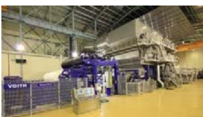
Dryer section of Siam Nippon Industrial Paper Co., Ltd.'s Yankee machine
