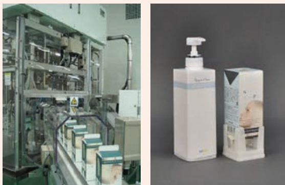
The specialized SPOPS filling machine (left) and product (right)
