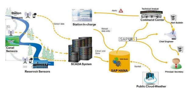
Flood Monitoring using data from structured data from SCADA systems and unstructured data like SMS/Text and Weather Maps
