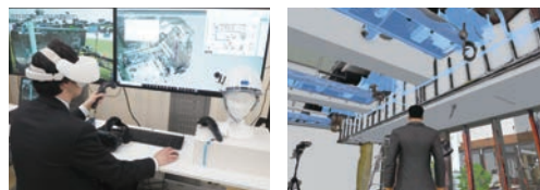
Installation drawings created by BIM are superimposed over VR images of the jobsite to verify progress and quality.
