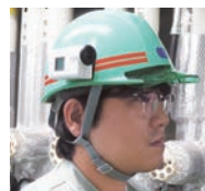
Camera images are used to create a virtual reality of the jobsite.
