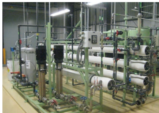
Filtration device using reverse osmosis membranes
