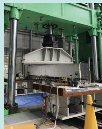
Load fatigue test using RC beam specimen
