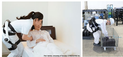
The robotic suit “HAL” is one example of a product that has been developed and produced for the nursing care field, as well as the plant floor. © Prof. Sankai, University of Tsukuba / CYBERDYNE Inc. HAL® is an exoskeletal suit developed and manufactured by CYBERDYNE Inc.
