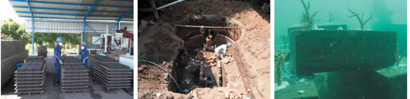
⚡ PT YTL Jawa Timur's FABAs paving block production (left), used in one of the 680 biogas units (center) and reef blocks (right) near the power plant
