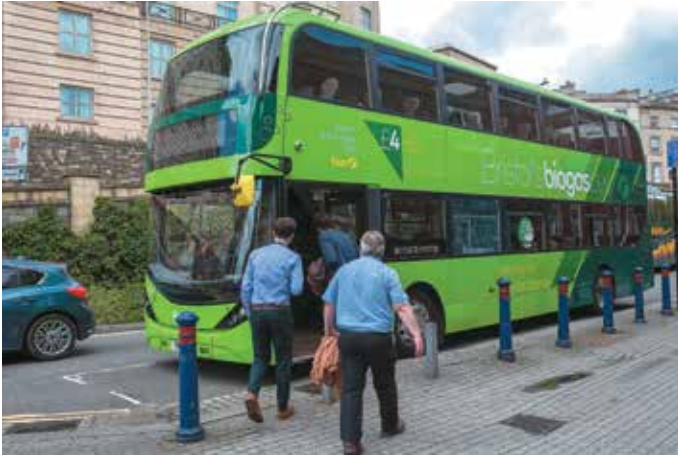
⚡ The “Bristol as a Future City” event tour bus seen here powered by biomethane derived from human excretion and food waste processed at GENeco UK’s anaerobic digestion plant facility in Avonmouth, Bristol, UK
