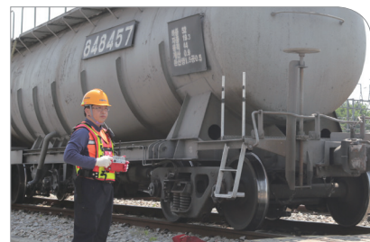
A KORAIL Employee Demonstrating Remotely Controlled Shunting
