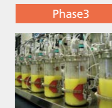
Corynebacterium used to convert and condense sugar solution into alcohol (isobutanol)
