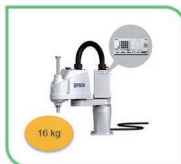
The T3 has a built-in controller
