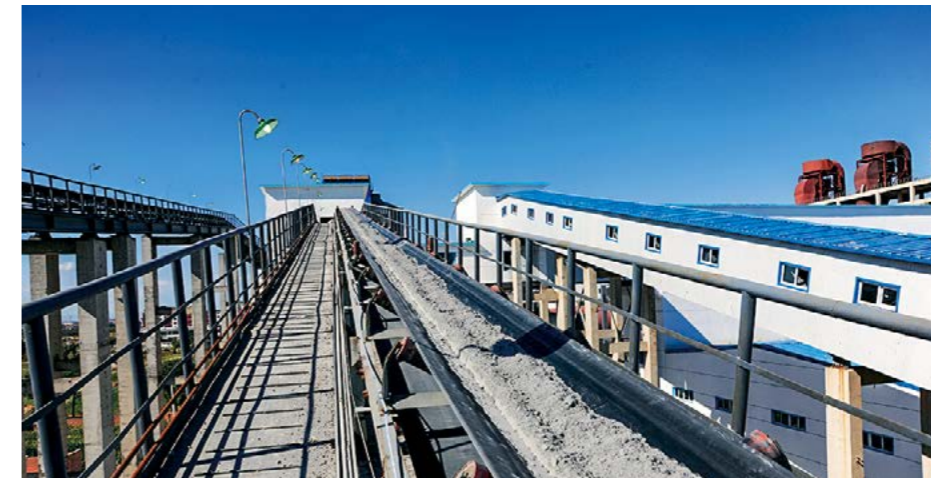
The High-aluminum fly ash conveyor of Datang Inner Mongolia Renewable Resources Company
