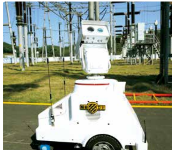
Robot of Zhaoqing Converter Station patrolling converter station equipment
