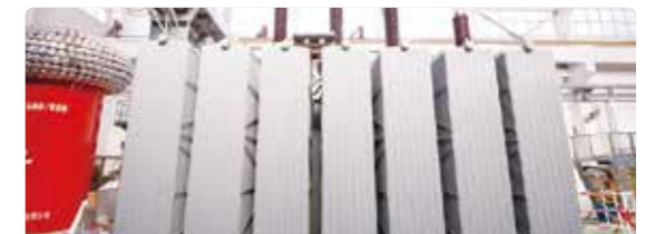
The country's first plant-insulated oil transformer was successfully developed in Guangzhou with each transformer saving nearly 20 tons of mineral oil per year.
