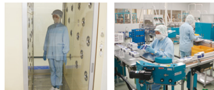
Measures for prevention of contamination by foreign matter (air showers) Visual inspection of products
