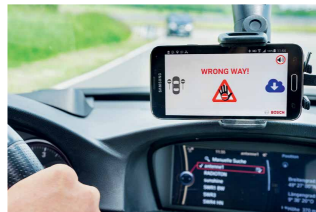
Bosch has developed a cloud-based solution that alerts wrong-way drivers and endangered drivers in the vicinity within ten seconds
