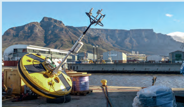
Buoys are used to collect metocean data for environmental purposes in Norway.
