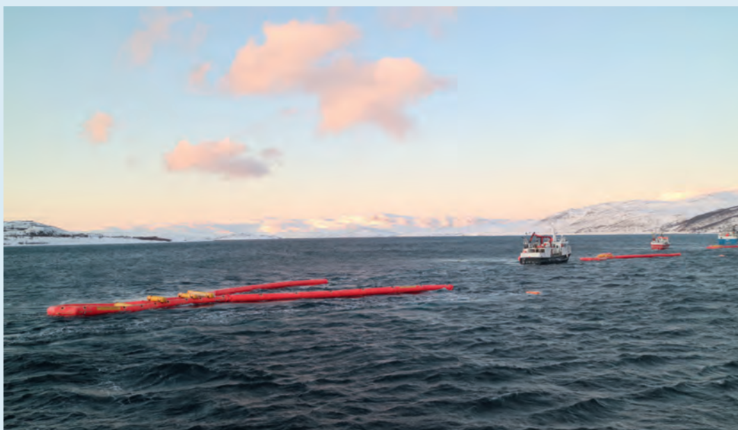
NOFO exercise in Repparfjord, Norway, January 2018. Local fishing boats take part in the exercise using the Current Busters barrier system to prevent oil slicks from reaching the shore.
