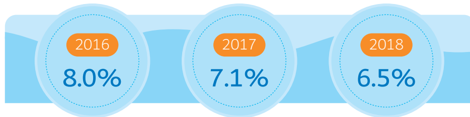
Graph: Annual Unaccounted For Water (UFW) As Percentage Of Total Water Supplied
