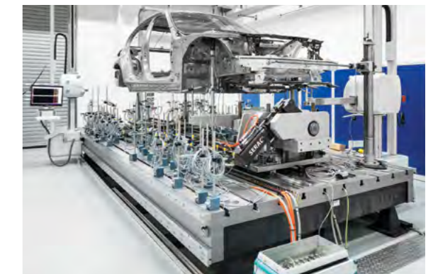
Torsion &amp; Bending Test Bench.
