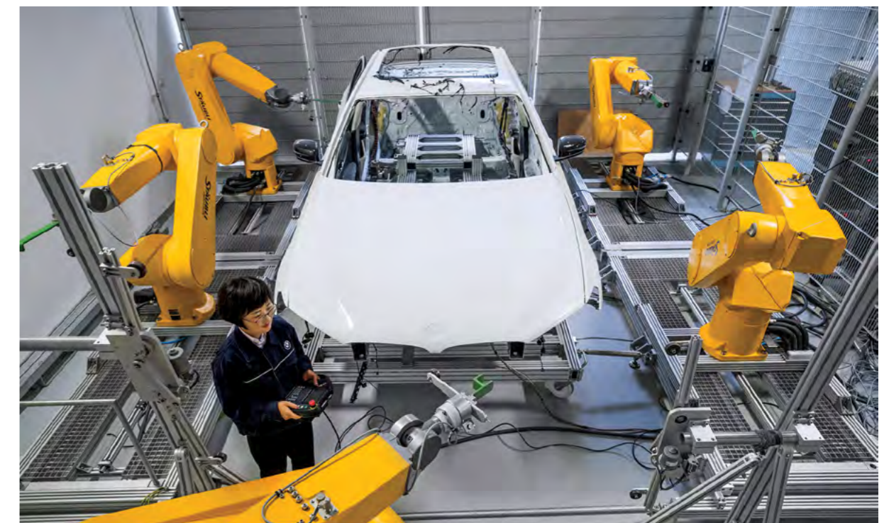
Car doors and flaps test bench in our R & D.
