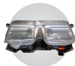
High Voltage Battery
