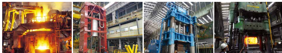
100-ton EAF 150-ton ESR 17,000 tons hydraulic forging press 4,200 tons press (max. 650-ton ingot)
