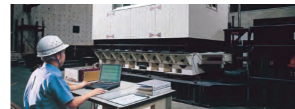
Experiment using a shaking table to test life-sized structures at a site that verifies seismic resistance levels
