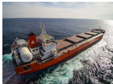
03 This LNG-fueled ship used POSCO's High Manganese Steel that can withstand temperatures as low as -196°C
