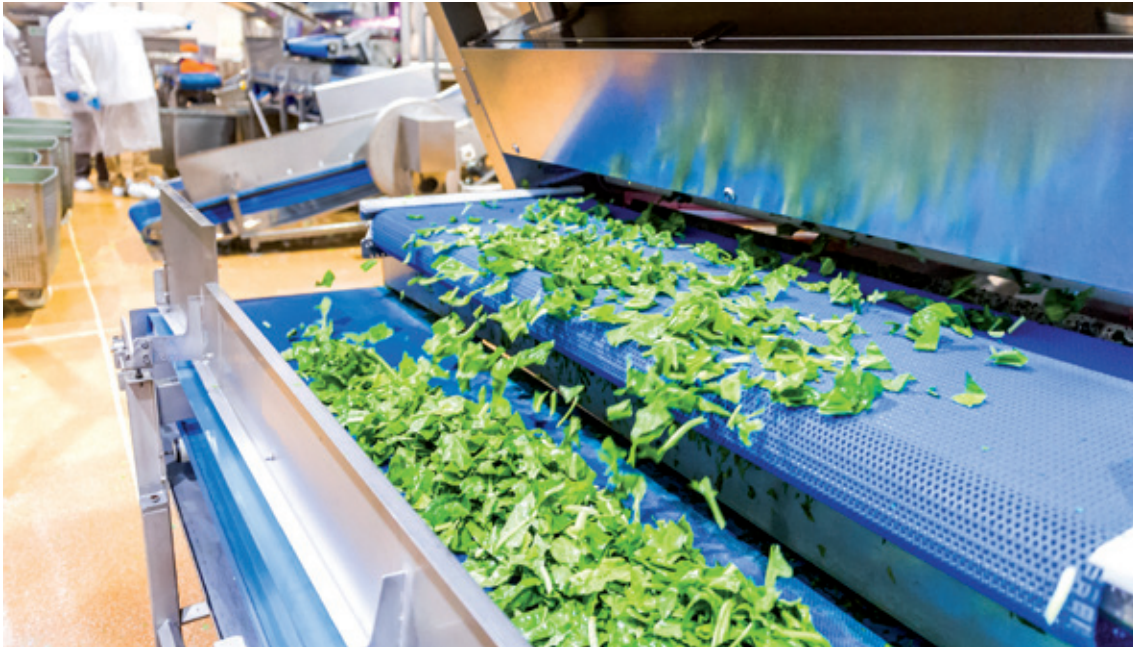
Artificial vision to monitor the process: our plants are equipped with artificial vision machines, cutting-edge technology that allows us to take 2,000 photos per second. This ensures the suitability and quality of all the leaves that pass through the conveyor belt. Should the artificial vision detect a leaf or anything of an inappropriate colour, it is expelled through a localized air jet, thus avoiding that the rest of the leaves in good condition are wasted.
