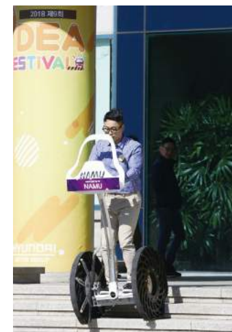
NAMU – the grand award winner in the 2018 R&D Idea Festival – implementing freedom in mobility by developing stair climbing wheels
