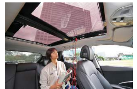
Performance evaluation of the second-generation roof panel
