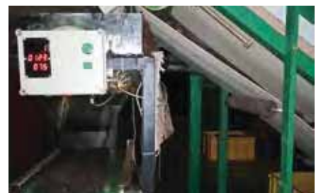
Automated dryer mouth weighing scale system
