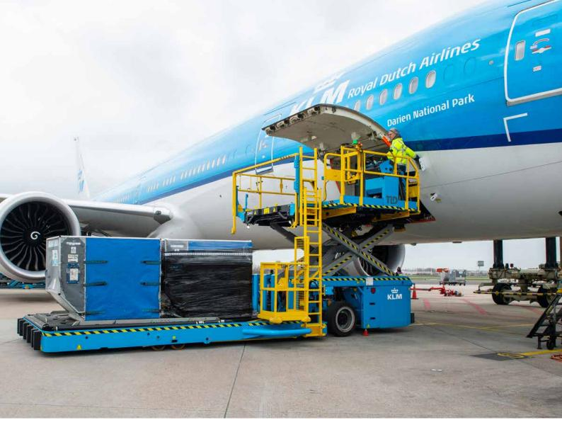
So back in 2016, KLM contacted several manufacturers of high loaders, a heavy-duty elevator that lifts cargo up to the belly of an aircraft. "We gave them our specs, they developed prototypes and we tested them on the ground to measure how it performed."
