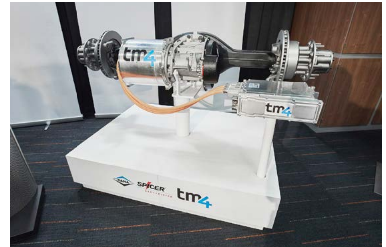
Dana axle with a TM4 SUMO electric powertrain (motor and inverter).
