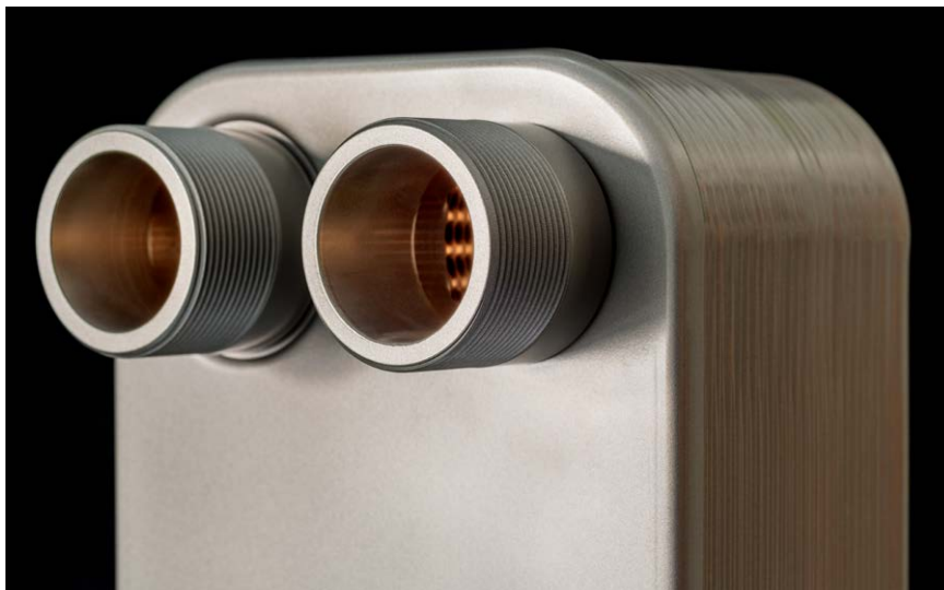
Two media at different temperatures flow on either side of thin plates and in opposite directions to each other resulting in heat transfer between the media.
