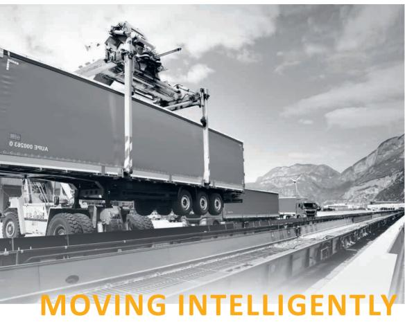
A semi-trailer is loaded onto the railway before crossing the Alps.
