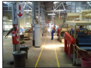
Photo 5: Inside one of the factories. Note the housekeeping, marked walkways, guarded machinery and fire extinguishers provision.
