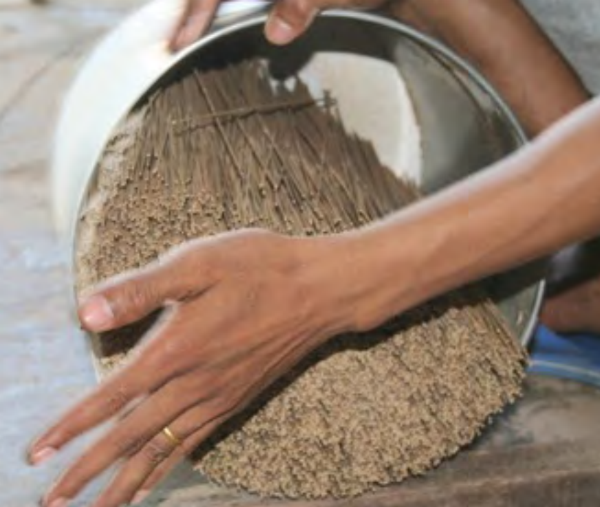
Homogenization of the sticks before drying.
