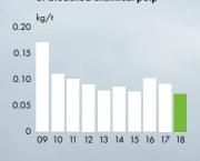
AOX indicates the amount of halogens bound to the organic compounds present in the effluent. The AOX load per tonne of bleached chemical sed by 57% over the last ter
