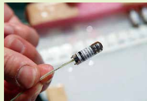
Archival electronic tags: The skipjack's daily swimming location and water depth, water temperature and skipjack body temperature can be recorded every 30 seconds throughout the year.
