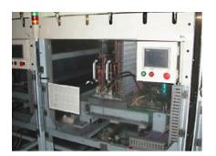
1. Air-tightness and pressure resistance inspection
