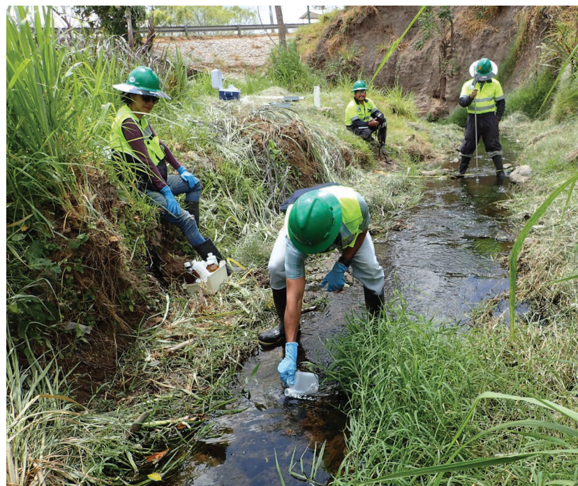
Measuring flow and taking water samples near Escobal Mine.
