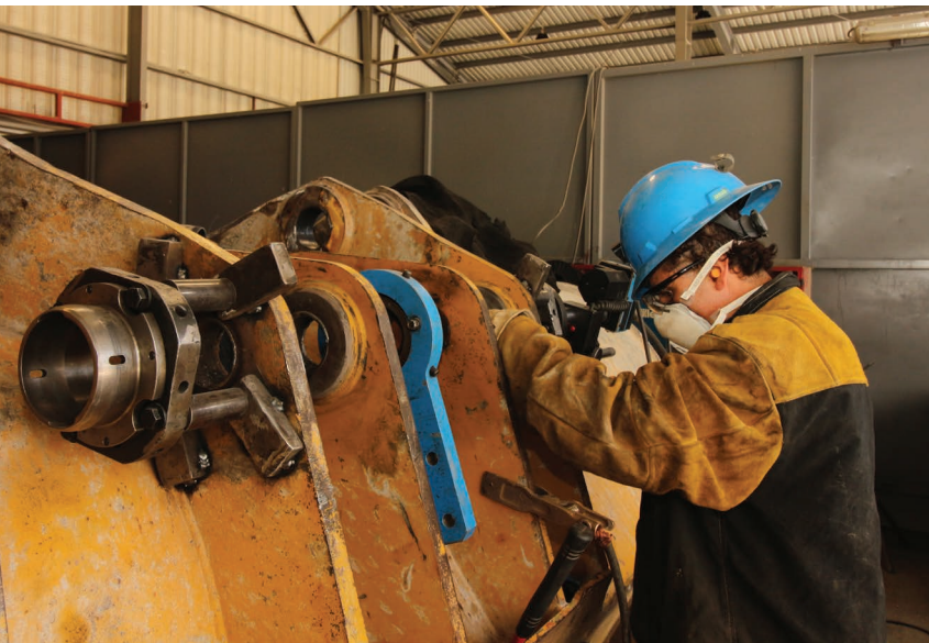
Maintenance inspection of underground loader bucket at MSR.
