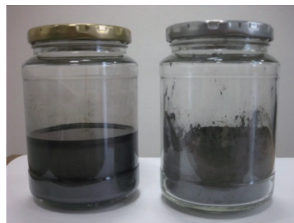
(Left) Notebook PC case (powder coating without using solvent) (Right) Normal solvent and powder coating
