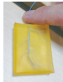
Reproducing the hollow structures of blood vessels makes it possible to simulate catheter manipulation Photo courtesy of Nagoya University School of Medicine
