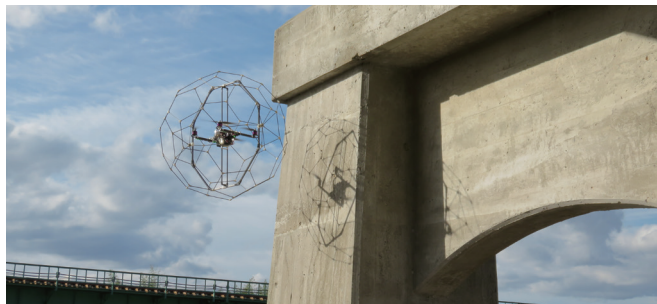
Checking bridge with spherical shell drone
