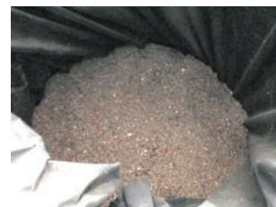
Copper pieces recovered from electric wire
