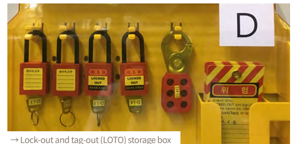
→ Lock-out and tag-out (LOTO) storage box
