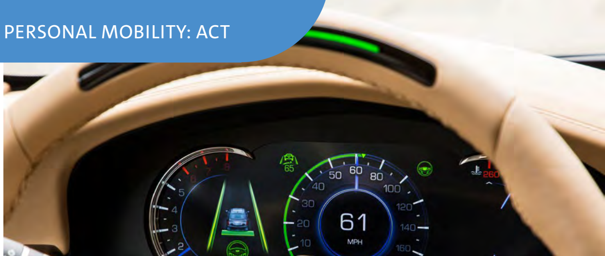
A steering wheel light bar and cluster icons indicate the status of Super Cruise™ and will prompt the driver to return their attention to the road ahead if the system detects driver attention has turned away from the road too long.
