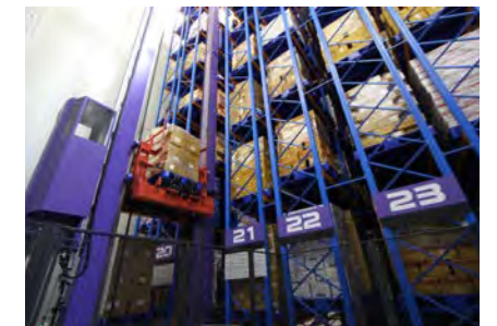
Automated freezer warehouse system delivered to a food product manufacturer in Thailand
