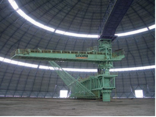
中材建设设计的水泥生产线技术装备：大型堆取料机 Technical equipment of cement production line designed by CBMI: Large stacker-reclaimer
