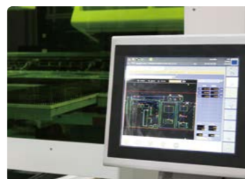
A fiber laser cutting machine is used to process components according to a nested design
