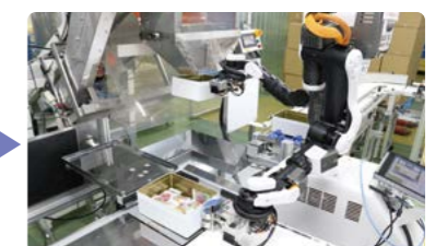
Based on the total weight, check the content amount and number of servings of crackers in the container. Forward to the next process only those that have successfully passed this phase.
