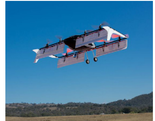
The Verti-plane prototype developed by AMSL Aero, a member of the muru-D SYD5 cohort.
