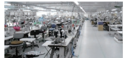
▲ The sewing floor has no pillars, allowing for the flexible layout of sewing machines
