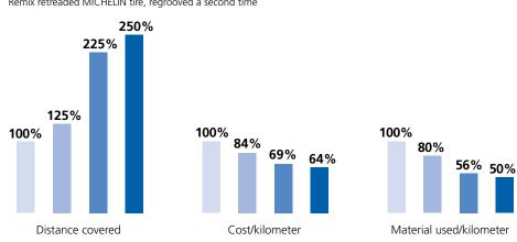
In other words, Michelin's retreading/regrooving solutions can keep truckers on the road 2.5 times longer on the same tire, or up to one million kilometers for certain long-haul tires with an initial lifespan of already 250,000 km. This offers three benefits compared with a non-retreadable, non-regroovable tire, whether premium or budget:
