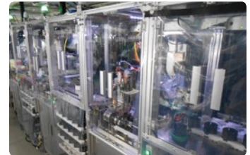
Automated lens barrel assembly equipment
