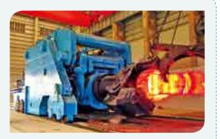
for invention, 9 patents for utility models and more than 30 published papers in science and technology. As the largest full-hydraulic forging manipulator in the world today, it marked the significant improvement of domestic production capacity of large and super-large forged piece and played an important role in supporting and promoting China's manufacturing of large forged piece and large forging equipment technology to surpass the world advanced level.
