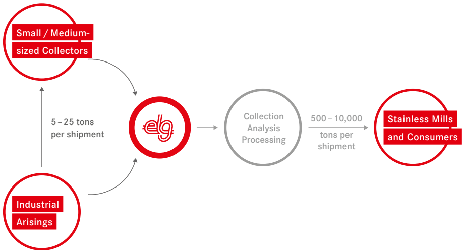
Figure 02 THE PROCESSING CHAIN IN METAL RECYCLING
