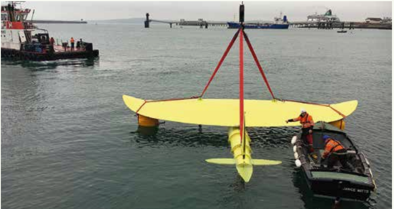
Minesto's Deep Green technology harvests low-flow tidal energy 15 meters below the surface
