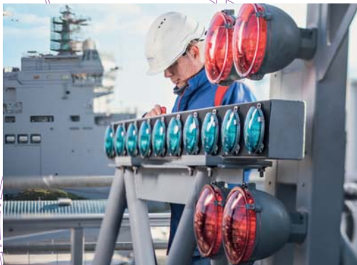
At Toulon, Éric supervises the positioning of a new deck landing mirror on the Charles de Gaulle aircraft carrier.
