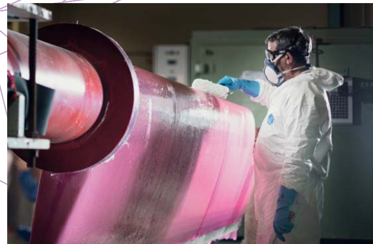
Patrick, experienced in working with composites, carries out the stratification of a rudder.
