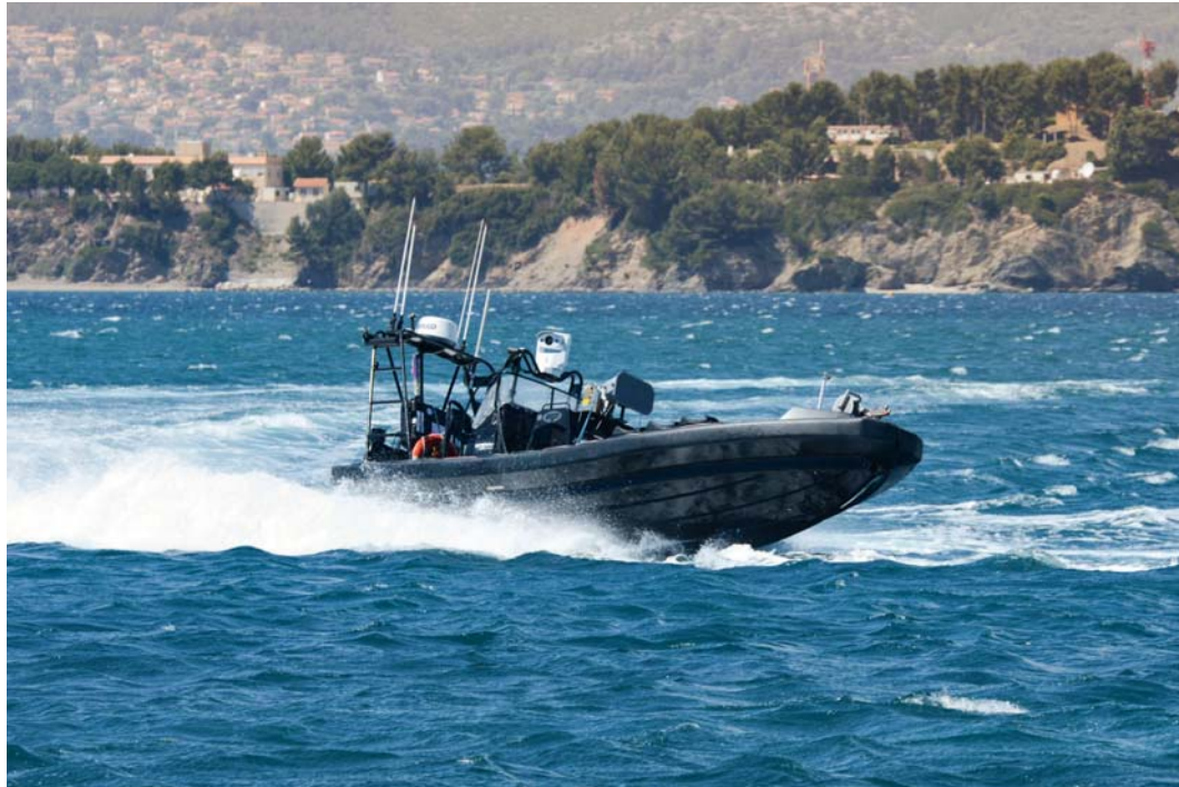
REMORINA, a surface drone developed by Sirehna, can approach an object independently or by remote control and interact with a threat.
