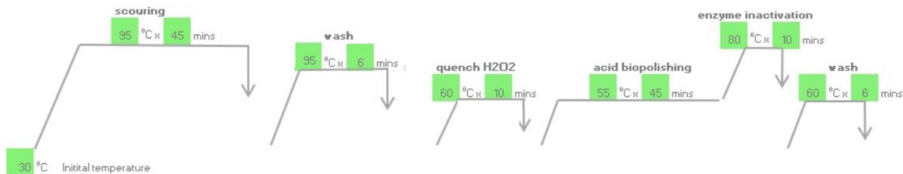
Figure 1: Working mechanism of the conventional process.
