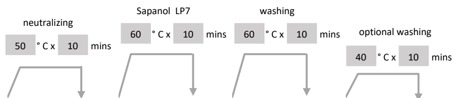
Figure 15: Working mechanism of the Sapanol LP7 sustainable low temperature soaping process.
